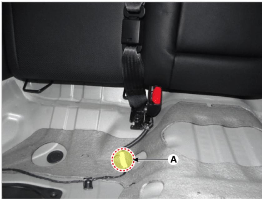
4. Remove the rear seat belt buckle (A) after loosening the mounting bolt.
