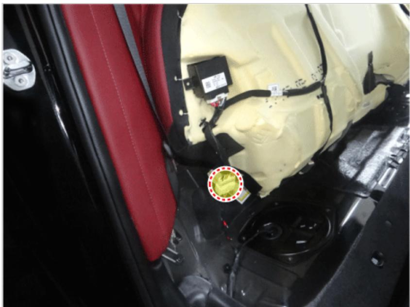
3. Disconnect the rear seat belt buckle connector (A).
